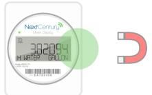
Configuration wireless communication initiated when a magnet is moved past the activation zone highlighted in this figure.
